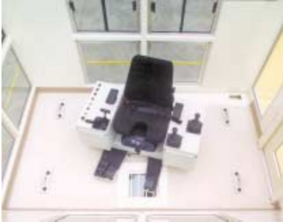
Outdoor gantry crane - US Steel Edgar Thompson Works. Slanted wall was designed by CID to reduce operator glare, improve visibility, and increase safety.
